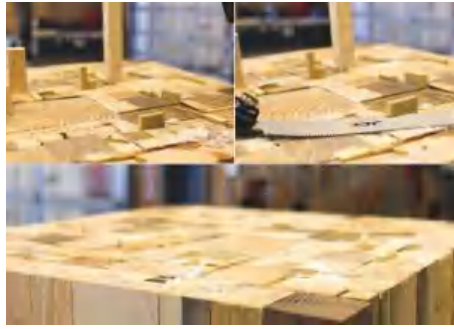
▲ Pic.4 First, fill any gaps with straight wood, then cut off any plug ends using a coping saw
